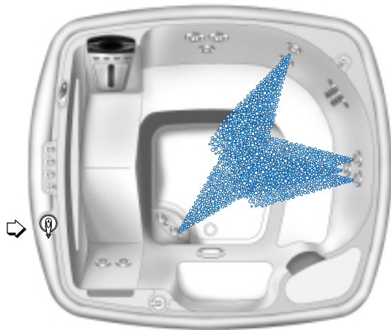
Left Jet Pump–Jet System 2 Left SmartJet® Lever in the 9 o'clock position
