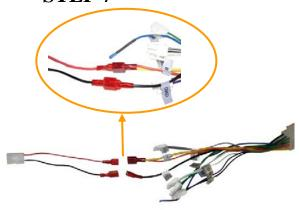
Join the Wire Harness Assembly and the Power Supply Adaptor together: **red to red** wire and **black to black** wire.
