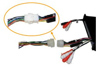
Connect the Amplifier Harness to the Wire Harness Assembly.
