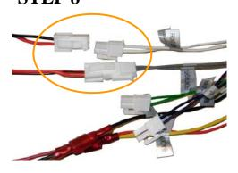
Join the speaker connectors to the left and right <u>front</u> connectors (gray and white wires) in the Wire Harness Assembly.
