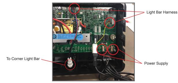
2. Disconnect the Light Bar Harness and Power Supply from the Control Box and Corner Light Bar.
