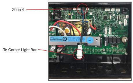
3. Connect the Direct Light Bar Harness to Zone 4 of the Control Box and the Corner Light Bar. Update Software Code. Replace control box cover and equipment compartment panel. Test for proper operation.
