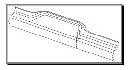
Cracks can occur on any part of the bartop. When this happens, the shell must be reinforced on the backside as well as the front side.
